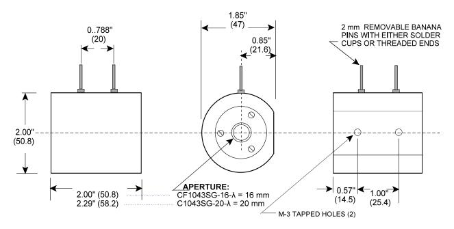
MODELS CF1043SG-16 & CF1043SG-20 LARGE APERTURE MODULATORS
