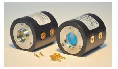
The CF1043 mechanical configuration yields the lowest capacitance devices for a given aperture size. This facilitates application to impedance matching with transmission lines, Blumlein structures, spark gaps, and solid state FET or avalanche transistor type drivers.
