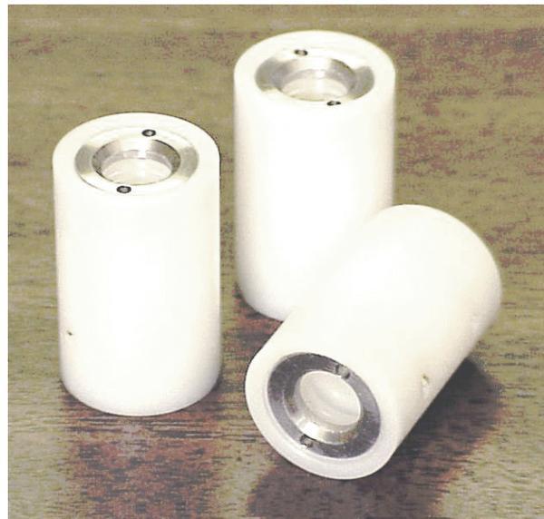
Sol Gel antireflection coatings are standard in the 1145 Series and are applied to the crystal for highest peak and average power applications. Sol Gel coatings are extremely efficient, having reflectance losses of 0.05%. Damage threshold for Sol Gel coatings is at least as high as that of the KD\*P crystal material at any optical fluence.
