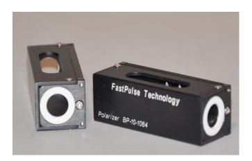
Plate polarizers with coatings provide very high extinction from single and double plate designs. BP Series standard polarizers incorporate 2 plates angled at 65° and mounted in a "V" orientation so there is no beam offset. Precision mounting methods insure stress free high performance.
