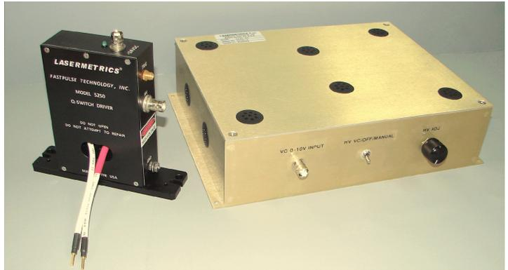
5250q-20 Laser Q-switch Drivers are valuable for laser Q-switching and cavity dumping. The drivers are effective in both intracavity and extracavity applications where a fast rise time pulse is needed. Typical rise times are < 5 ns. The drivers provide the latest technology in reliable, solid state, high voltage switching design
